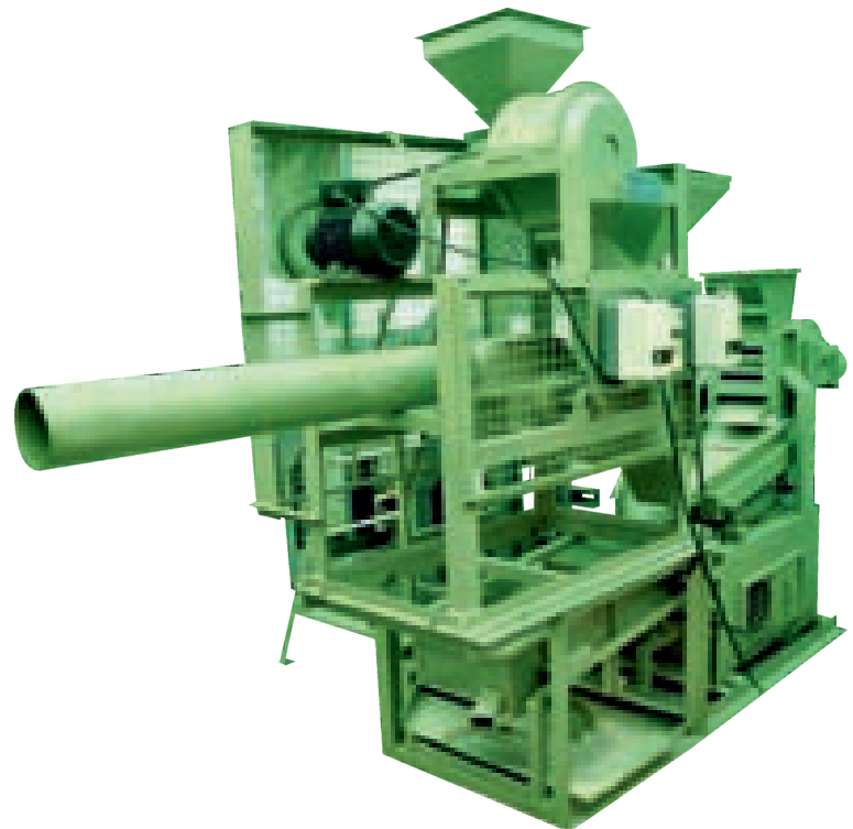
Fig. 5: Small millet destoner, grader cum dehuller
